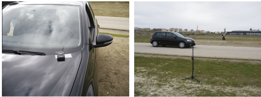
Fig. 9. The body-pack transmitter for the embarked wireless system of the rolling microphone (left) and the far-field microphone for measuring the pass-by noise (right).
