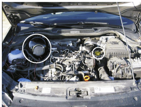
Fig. 7. Position of the spherical source and microphone inside the engine hood (left), and the external hemispherical distribution of microphones (right) for the determination of the engine hood Transmission Loss.
