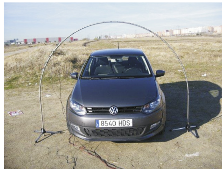
Fig. 7. Position of the spherical source and microphone inside the engine hood (left), and the external hemispherical distribution of microphones (right) for the determination of the engine hood Transmission Loss.
