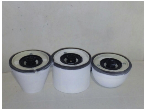
Fig. 2. Show the three bases glued together with the speaker's base and the speaker joined. In the outer part of the base one plastic strip was placed for acoustical isolation.
