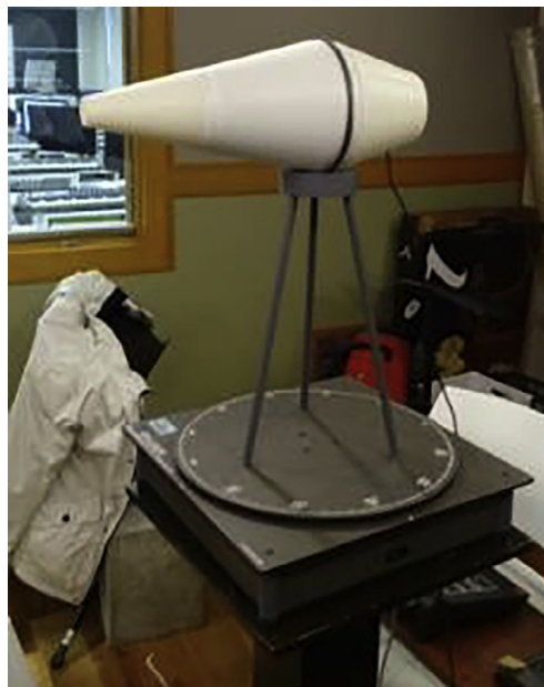
Fig. 4. Sound source mounted on the turntable.
