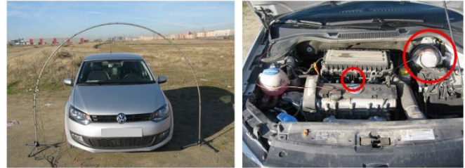
Figure 6. Positions of the loudspeaker and microphone inside the engine hood (right), and position of the microphones outside in the first 5 positions (left)
