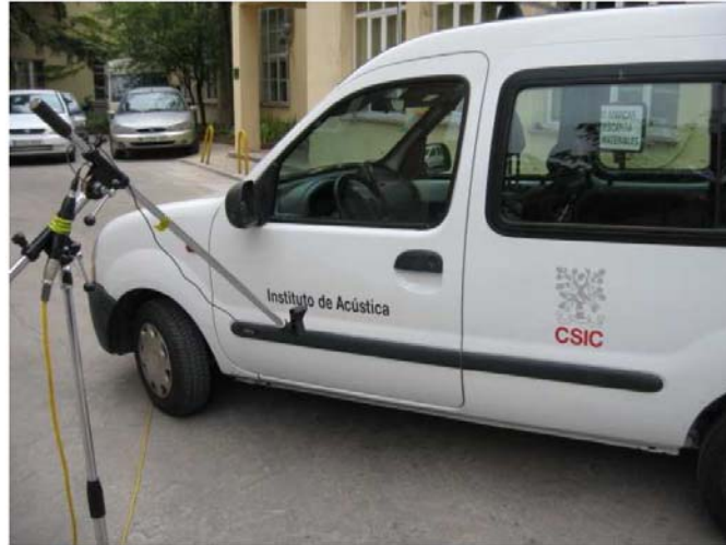
Figure 4 Position of the outside, lateral microphone m_3 (see online version for colours)
