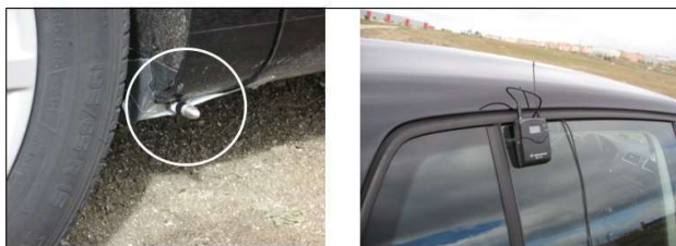
Figure 8. Position of the microphone near the rear tire opposite to the exhaust pipe (left), and position of the body pack transmitter (right).
