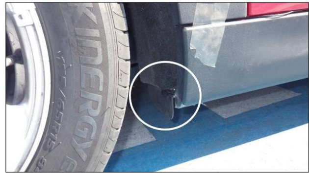
Figure 2. Position of the rolling microphone close to the rear wheel for the rolling noise measurement.
