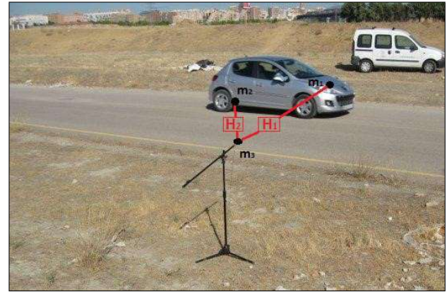
Figure 11. Measurements of noise in the near and far fields of a vehicle.
