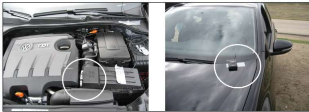
Figure 7. Position of the microphone inside the engine hood, close to the air intake system (left), and position of the body pack transmitter (right).
